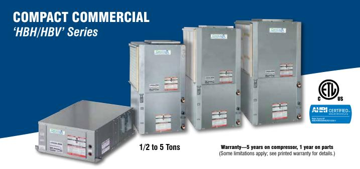
Individual HB Series units are connected by a water loop which allows heat transfer throughout the building. Excess heat energy is rejected through a cooling tower; additional heat energy is added by a boiler in the loop.
